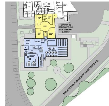
12 Renovate part of comm ctr - integrate into library
