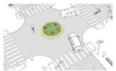
**Mini Circles** are installed in the middle of an intersection to slow down cars passing through. They function like a small roundabout.
