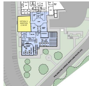
11 Construct addition in courtyard
