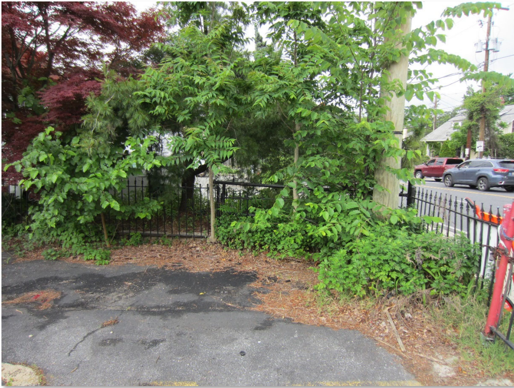
Picture 1 – Intersection Sight Triangle from Proposed Driveway Blocked by Vegetation on Adjacent Lot
