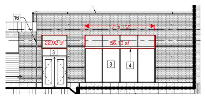
2. **Description of Alternative Concept:** Eliminate the upper section of windows and associated sunshade and replace with brick veneer.
