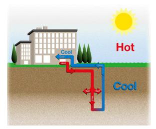
Heat pumps, installed on the lower level, convey heat to and from the earth through a geothermal ground loop system. The geothermal system uses water in a closed loop/recirculating arrangement and transfer building heat to and from the ground. The geothermal system acts as a storage of heat.
