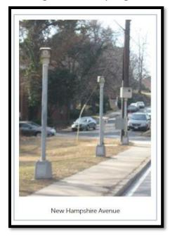
Automated speed enforcement (speed cameras) is a less commonly used form of automated enforcement used to address vehicle speeds, automobile collisions and speed related injuries. Speed cameras detect the speed of motor vehicles and photograph vehicles exceeding a preset speed threshold. Jurisdictions use speed cameras to supplement traditional speed enforcement programs. The use of automated speed enforcement does not eliminate the need for personnel. In particular, automated speed enforcement
