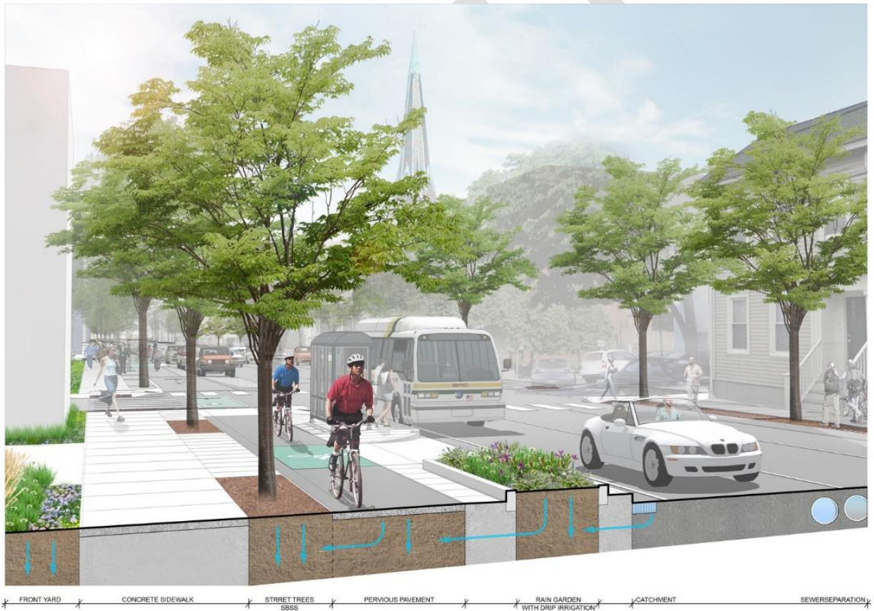
Figure X: Potential Stormwater Treatment within the Right-of-Way
