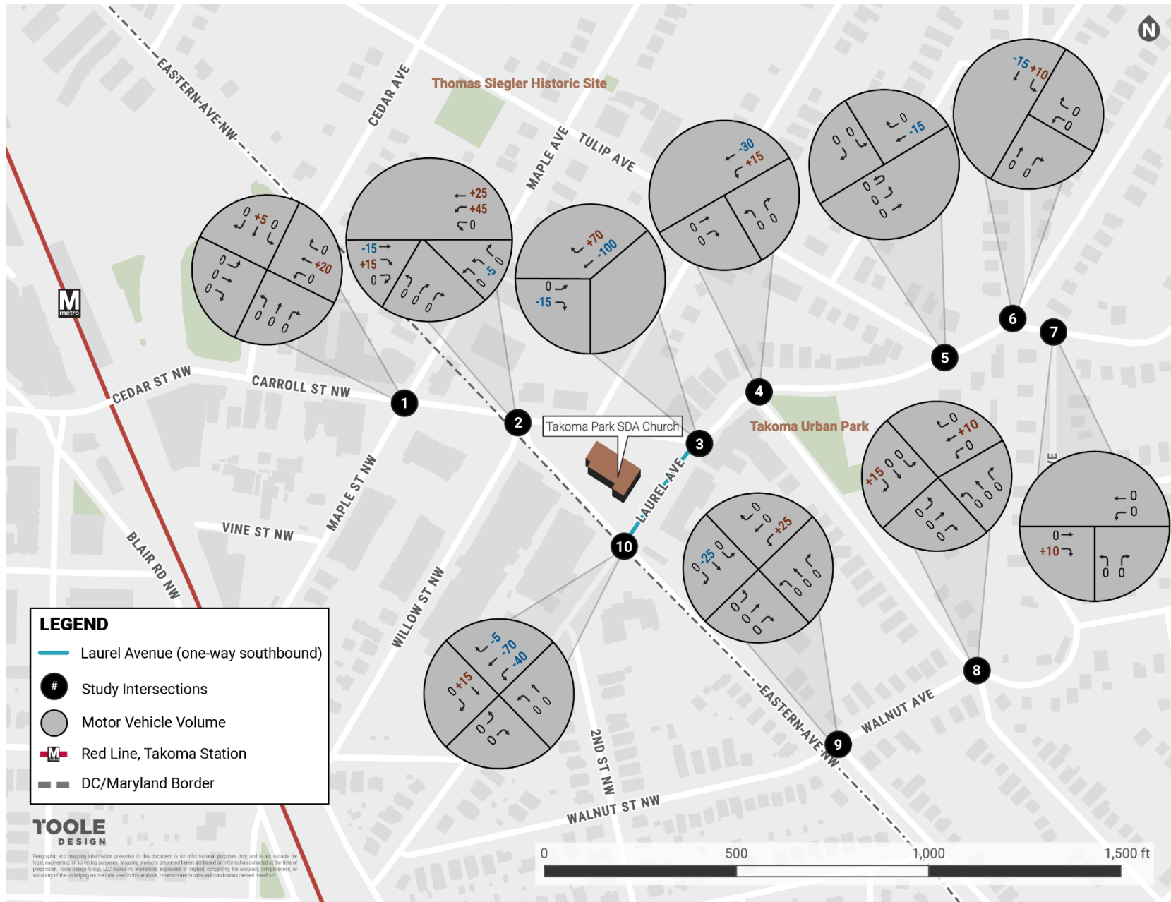
Figure D- 5: Change in Turning Movement Counts between Baseline and Reroute Scenario – PM Peak
