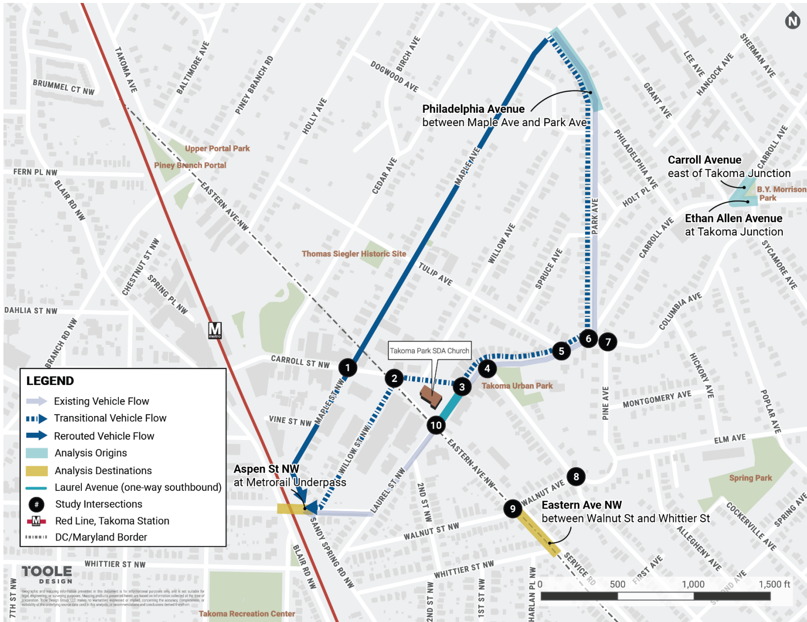
Figure C-1: Existing, Transitional, and Reroute Scenario Vehicle Flows from Philadelphia Avenue to Aspen St NW
