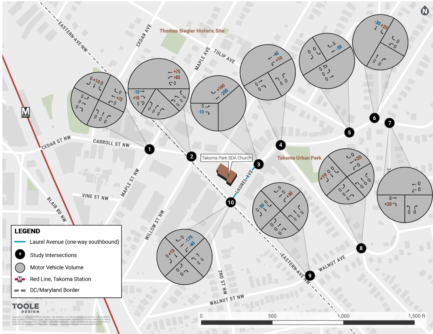
Figure D- 2: Change in Turning Movement Counts between Baseline and Reroute Scenario – AM Peak
