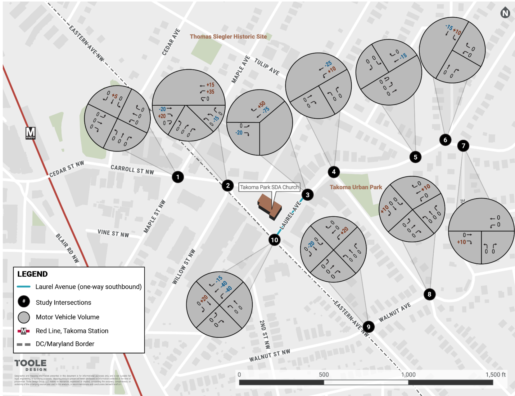
Figure D- 8: Change in Turning Movement Counts between Baseline and Reroute Scenario – Sunday Peak
