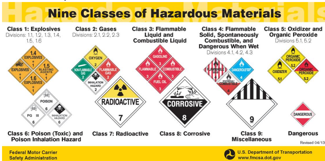
Figure 80: Placards used for the nine classes of hazardous materials as defined by US Department of Transportation
