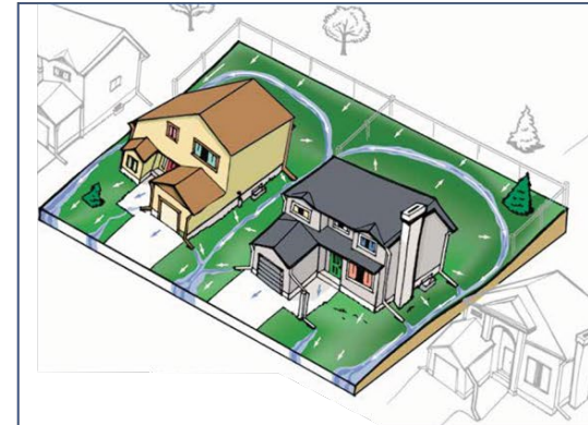
Grading can be used to maintain positive drainage without directing runoff to neighboring properties. Image Credit: City of Edmonton, AB, Canada Image may not be reproduced without permission
