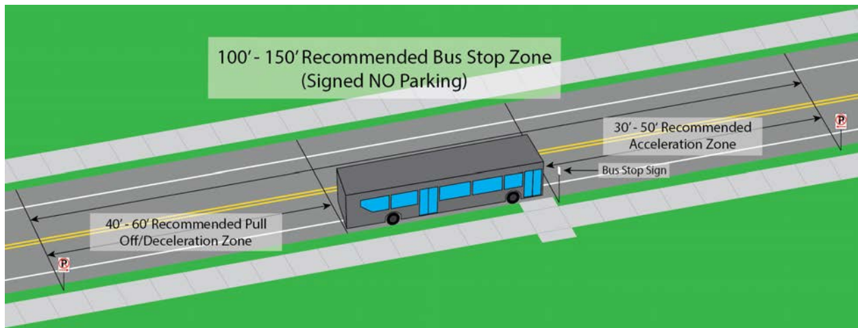
Figure 3-5: Mid-Block Bus Stop Design Considerations
