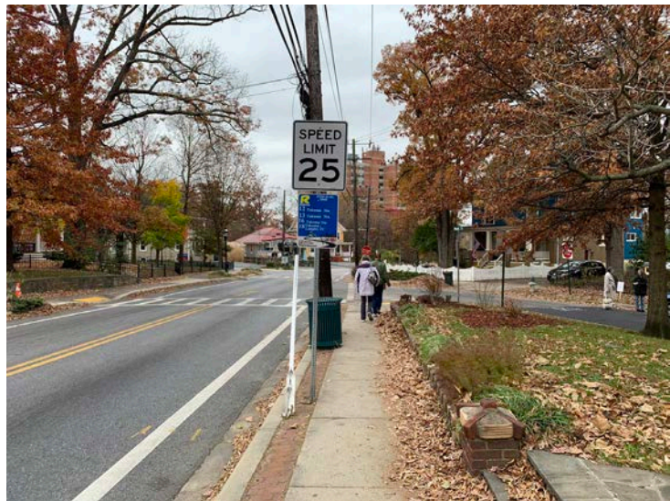
Figure 2-7: Narrow Sidewalks are a Leading Cause of ADA Non-compliance
