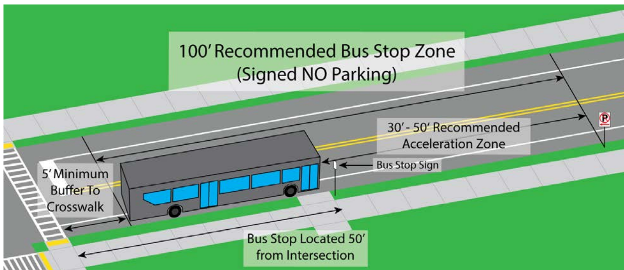
Figure 3-4: Far-Side Bus Stop Design Considerations
