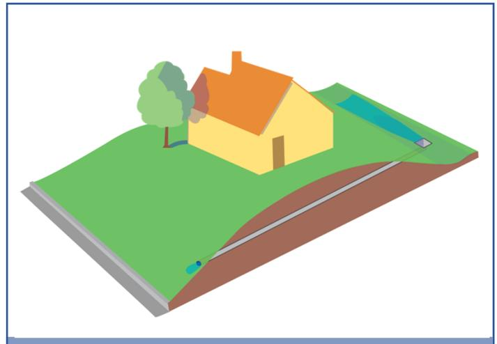
Private storm drain systems can be used to direct water when grading cannot.
