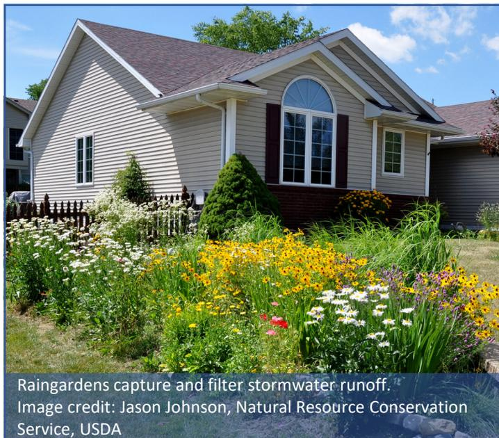
Raingardens capture and filter stormwater runoff.
