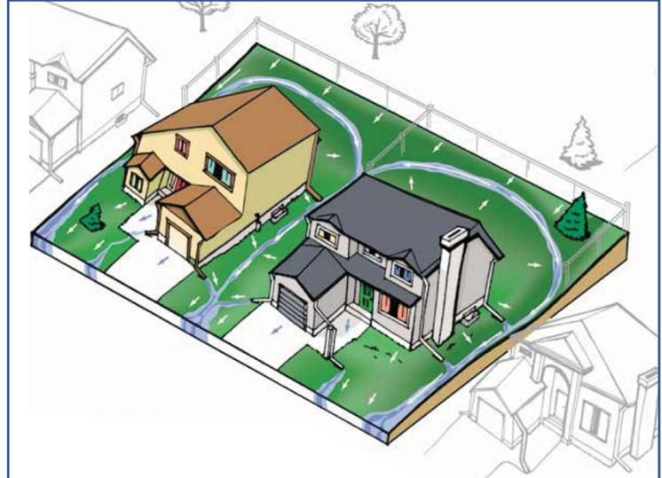
Grading can be used to maintain positive drainage without directing runoff to neighboring properties.
