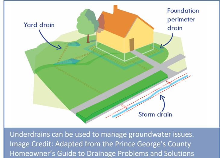
Underdrains can be used to manage groundwater issues. Image Credit: Adapted from the Prince George's County Homeowner's Guide to Drainage Problems and Solutions
