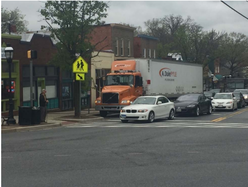
Photograph shows a WB-62 semi-trailer sitting half in the intended area with the rear of the trailer out into the southbound right turn lane to westbound Carroll Avenue. There is a UPS delivery truck sitting behind the semi-truck. During the morning peak, this creates delays for southbound traffic flow.
